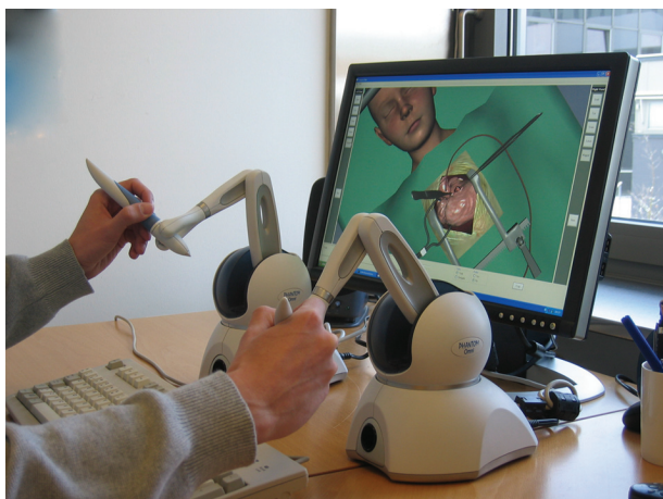
Fig. 1. Surgical simulation. Two Phantom Omnis (Sensable Technologies, USA) are used for free-hand interaction with force feedback. Cutting and tissue manipulation can be performed interactively.
