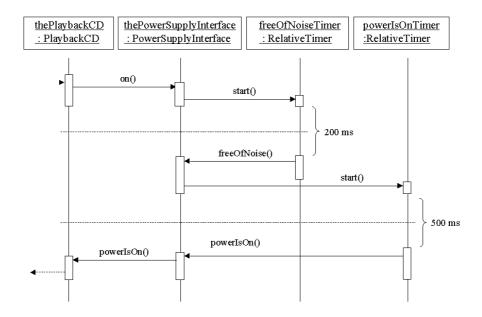
Figure 8: Interaction diagram for PowerSupplyInterface::on
