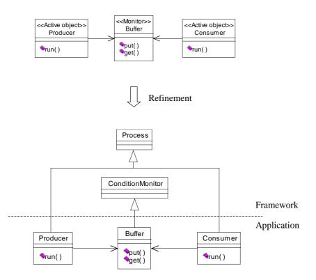
Figure 4: Refinement from design level modeling to technical design
