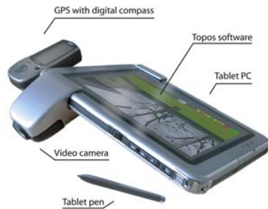
Figure 1: The SitePack appliance is assembled from off-the-shelf hardware components, consisting of a tablet PC with a pen input device, 1GHZ processor, 512 MB RAM, and a 16MB graphics card. The external devices are a 640 x 480 pixel web cam integrated in a bracket mount, and a GPS with digital compass.
