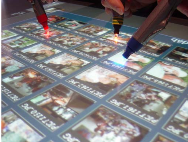
Figure 6 The MultiLightTracker technique in use on a MediaTable
