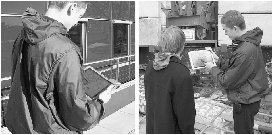
Figure 4 Context-aware hypermedia on a mobile tablet PC with camera [SitePack (Nielsen et al. 2003)]. The tablet has network connection through a Bluetooth- and GRPS-enabled cell phone and reads GPS coordinates from the GPS unit visible in the user's pocket (b).
