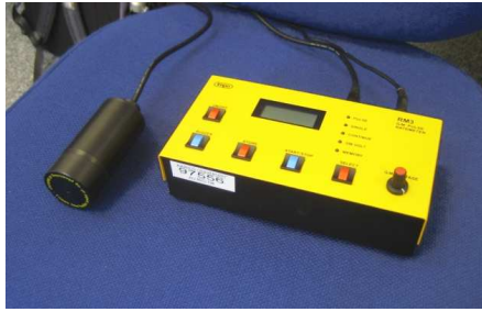
(a) Geiger-Müller tube in holder (left) and pulse ratemeter with data log and serial interface (right)
