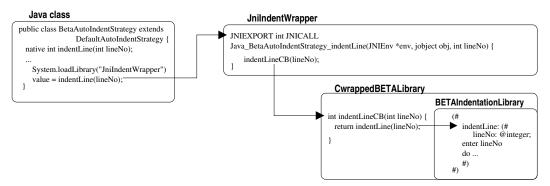
Fig. 1. Java BETA interoperability using JNI
