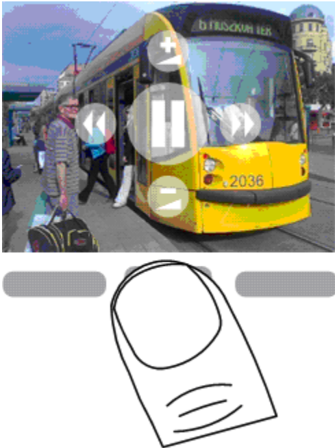
Figure 1. Function preview graphics on screen when a finger is resting on the navigation key.
