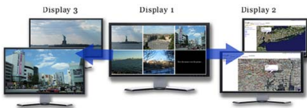
Figure 1. An example of a multi-display setup with an overview display, a display showing the location of the photo and a display showing the photos in full resolution.
